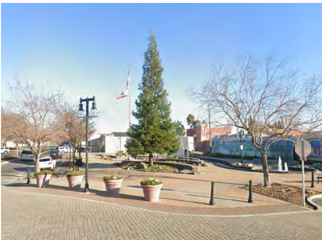
Curb extensions and wide sidewalks at Santa Fe Street and 3rd Street help to reduce motor vehicle traffic speeds in Downtown Riverbank. Photo: City of Riverbank
